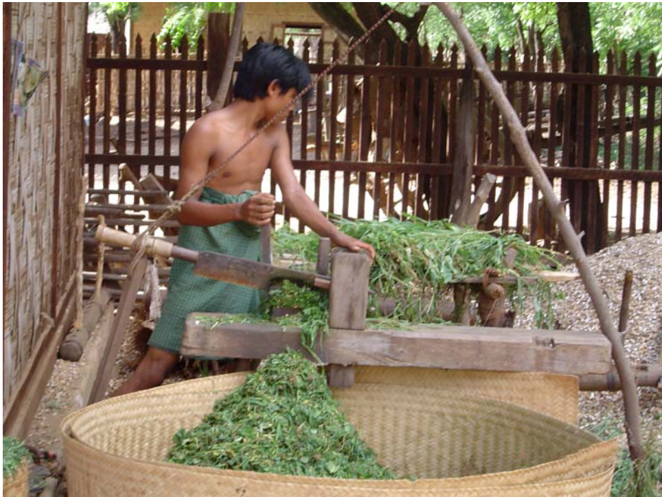
Figure 2.5 Chopping grass and straw using a homemade cutter
