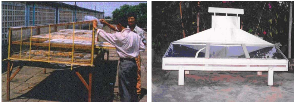
Figure 2.1: samples of solar dryer - solar cabinet dryers (Cheapok & Pornnareay 2005) and solar box dryers (Gewali, Joshi & Ramchandra 2005).
