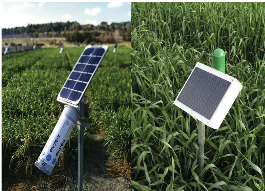
Fig. 1 – Custom developed ArduCrop wireless infra-red canopy temperature sensor (left) and ArduCrop dry reference sensor (right). The ArduCrop dry reference sensor comprises two infrared thermometer sensors (MLX90614-BCF from Melexis, Ypres, Belgium): 1) a downward-looking sensor to measure the canopy temperature (obscured) and; 2) an upward-looking sensor mounted inside a green hemispherical dome made of plastic, the dry reference. (For interpretation of the references to colour in this figure legend, the reader is referred to the web version of this article.)
