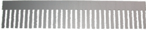
Figure 7: Practically waste-free sheet metal cut-out with identical width of tooth and slot
