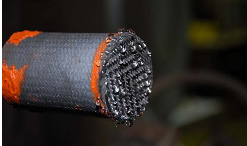
Figure 10. Second test assembly during water cooling supply check.
