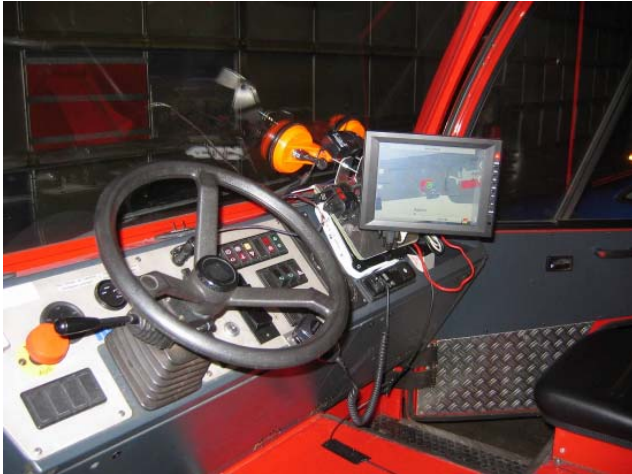
Figure 3. luggage car with integrated onboard unit
