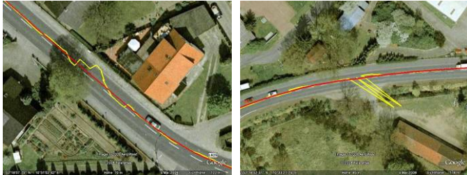
Figure 8. Comparison of single GPS and integrated position solution [6]
