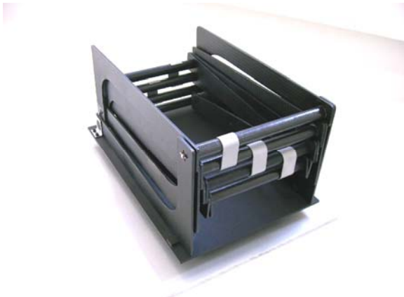
Fig. 4. Boom links in stowed configuration (still without mechanisms, and locked with aluminium clamps)
