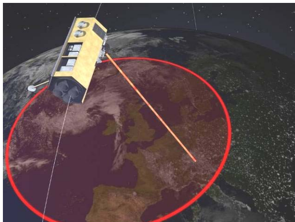
Figure 1-1: Illustration of a down-link from the Earth observation satellite TerraSAR-X to an optical ground station at DLR Oberpfaffenhofen.
