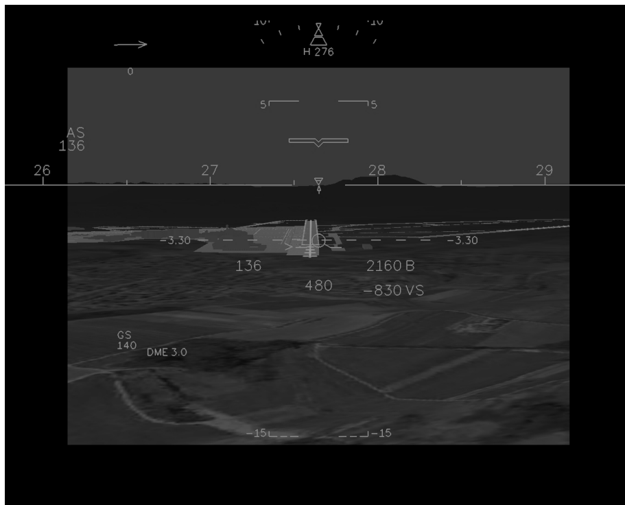
Fig. 3: EVS Head Down Display with EVS image and guidance symbology including Flight Path Vector and Flight Path Angle Reference Cue
