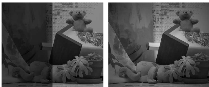
Fig. 11. Examples of local scaling of intensities with s_1 = 0.3 and s_2 = 0.7 (left) and linear down-scaling from image center with s = 0.5 (right).
