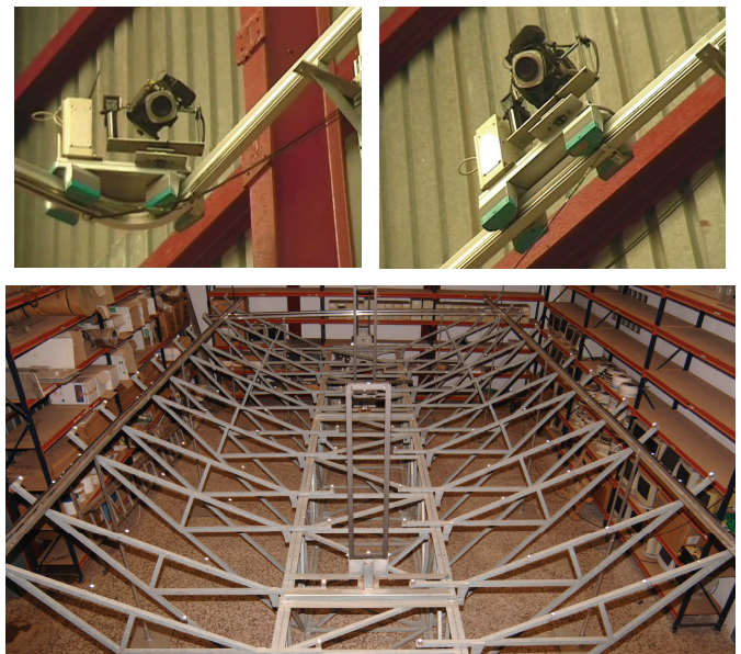
Figure 3: Camera shuttle in different measuring positions (top), and space frame with targets on cantilever arms and receiver supports (bottom)
