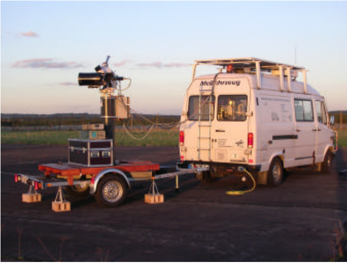
Fig. 1 In 2004 the Transportable Optical Ground Station in a downlink from a tethered balloon in the UK.
