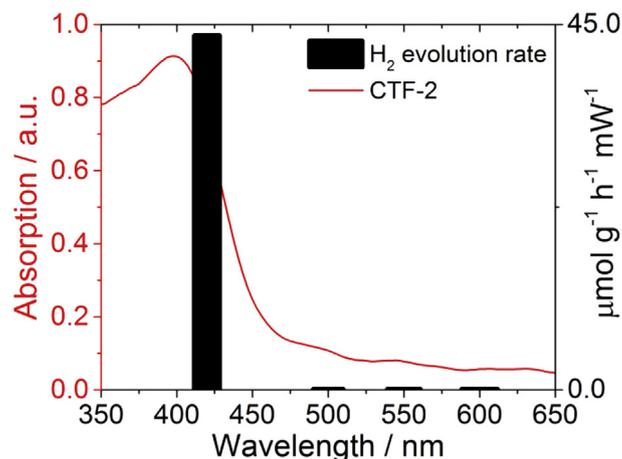
Fig. 4. Wavelength dependency of the photocatalytic hydrogen evolution for CTF-2 ball milled using band-pass filters (420 nm, 500 nm, 550 nm and 600 nm  $\pm$  10 nm, FWHM). The suspension of the polymer in water with 20 vol % of triethanolamine and 3 wt % Pt was measured in a quartz cuvette with an area of  $7.8 \text{ cm}^2$  for an illumination time of at least 5 h.
