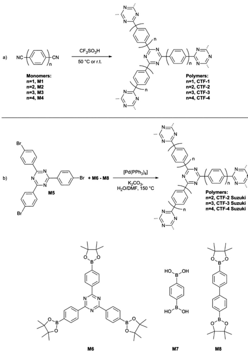
**Fig. 1.** Synthetic scheme for covalent triazine-based frameworks (CTFs) showing their representative repeating units: a) Trifluoromethanesulfonic acid catalyzed cyclotrimerization and b) Suzuki-Miyaura type polycondensation. Note that these simplified schematic representations do not show the defects and end-groups that will be present in these amorphous, porous networks.
