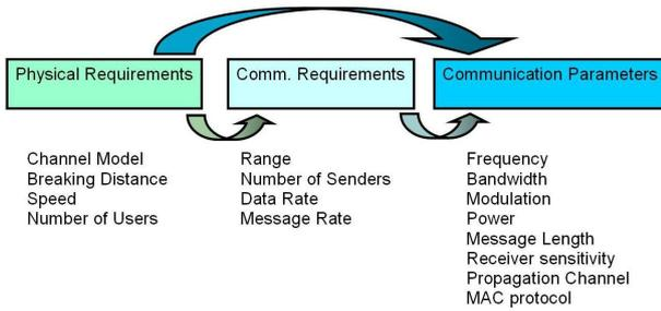
**Figure 1: Relationship between physical requirements, and communication parameters.**
