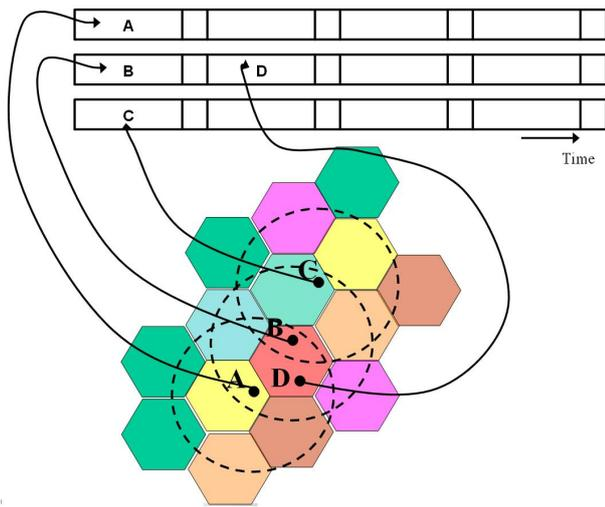
**Figure 4: Cell-based Orientation-Aware MANET Broadcast (COMB) Protocol. A MAC layer protocol suitable for railroad purposes.**
