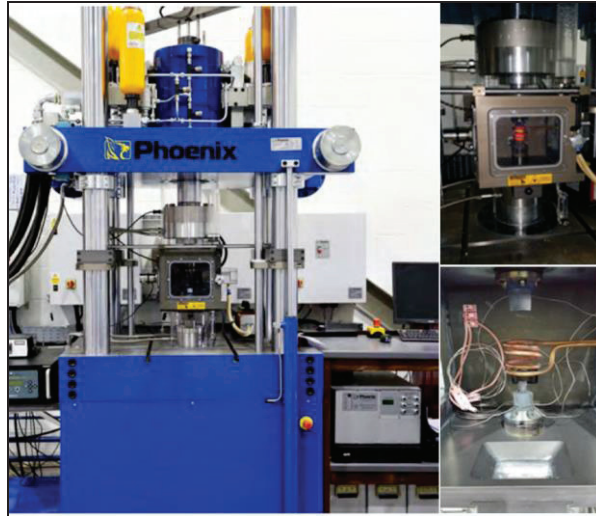
FIGURE 1. Servo-hydraulic forging simulation machine, chamber and interior
