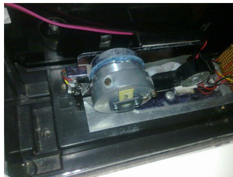
Figure 9 A miniaturised dosimeter in the spectrophotometer prior to being measured
