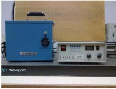
Figure 10 Solar simulator that provides an artificial source of UV radiation.
