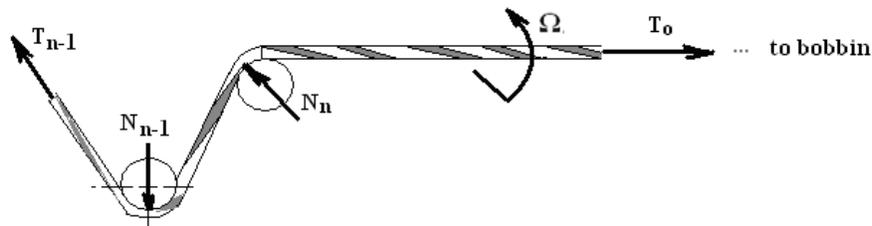
Figure 7 A schematic of the twist zone and final part of CERS showing the twist insertion.
