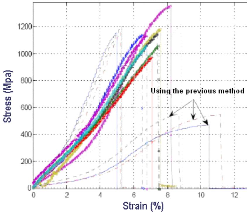
Figure 11 Stress-Strain curves of CNT yarn spun from the same drawable forest using the previous and modified processes: A comparison of the tensile strength of the CNT yarn samples spun from two methods.
