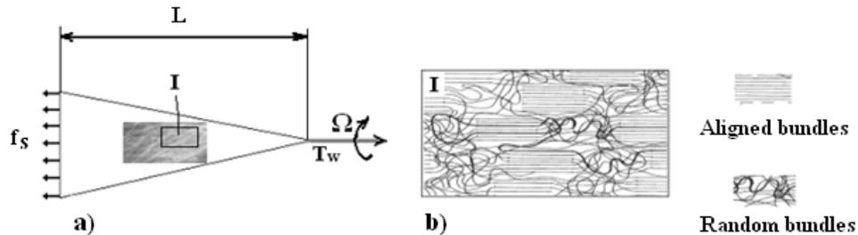
Figure 5 A model of CNT web structure.  $L$  is the length of CNT web.
