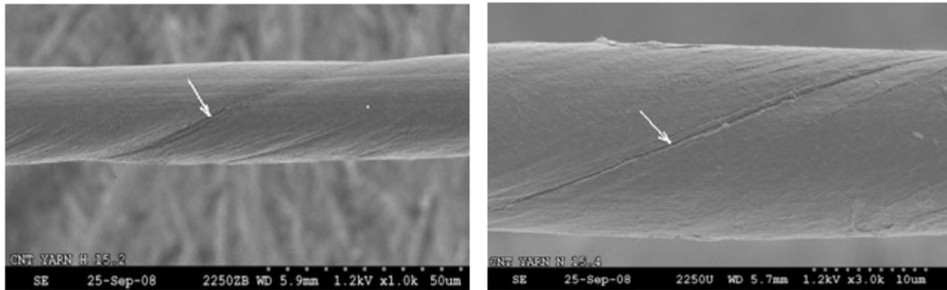
Figure 9. Micrograph (SEM images) of the surface layer for MWCNT yarn using the modified process: (a) yarn from web treated at 200°C and (b) yarn from web treated at 400°C. Arrow on the images shows the twist angle of yarn.
