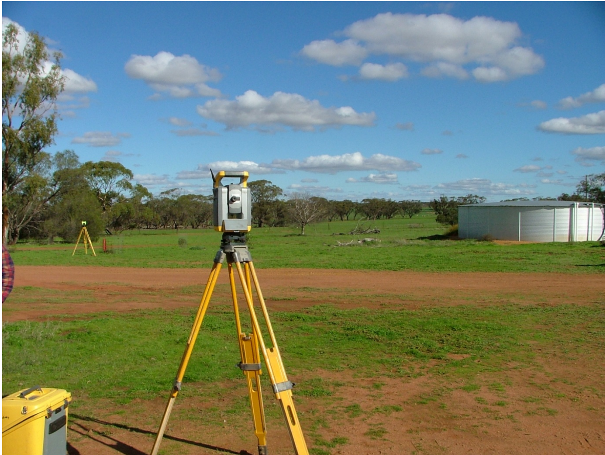
Figure 9: Trimble S6, with resection control point and galvanised steel tank in background.
