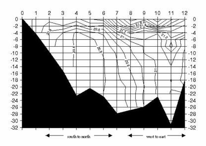
Figure 4: Survey day 1 locations, (a) temperature (°C) and (b) salinity profiles recorded on September 20, 2004. Locations are about 5 nautical miles apart. Changes in the predominant direction of the cruise track are indicated at the bottom of the panel.
