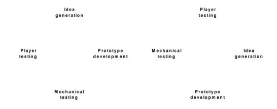
Figure 11.1 - Design cycle. Left: Traditional, player testing occurs after prototype development; Right: Modified, player testing is the starting point for idea generation.
