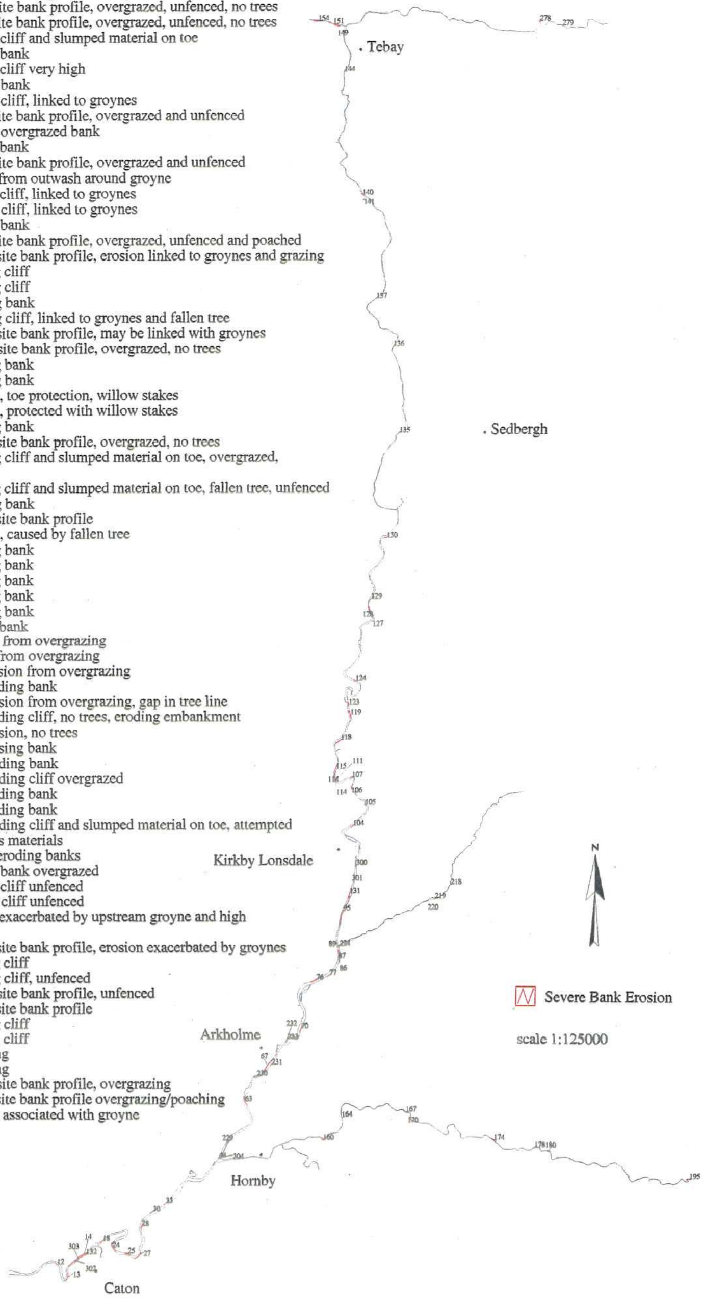
Figure 5.15 location of severe bank erosion
