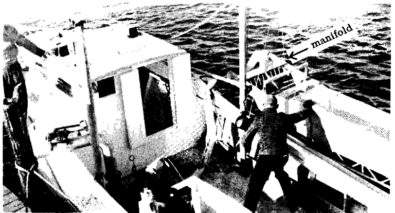
Plate 2. Lowering the hydraulic clam dredge.
