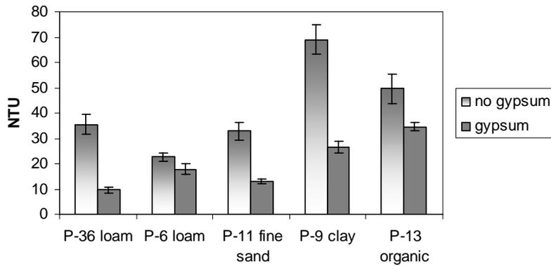
Figure 3. Turbidity of leaching waters from soil columns with and without gypsum. See caption of Figure 2 for more details.
