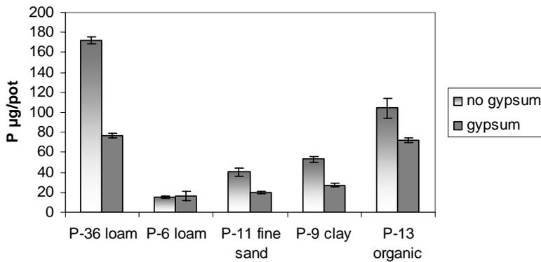
Figure 2. P-leaching from ½ kg soil columns treated with 2 g gypsum or not. Soils originate from fields of different soil type and P-status. Numbers represent soil test-P (mg/l soil, with acid AAC extraction). The bars represent cumulative ortho-P concentrations after 4 leaching procedure by 300 ml water. Columns were not fertilized.
