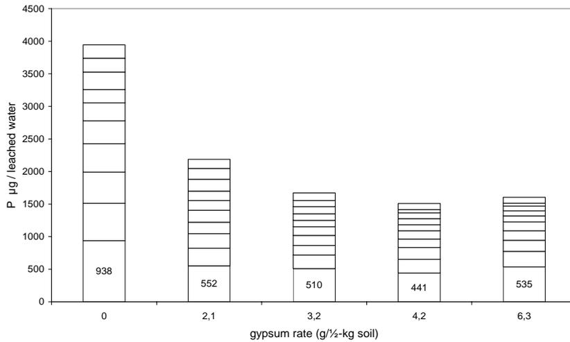
Figure 1. P-leaching from ½ kg soil columns treated with 0-6.3 g gypsum. Numbers represent ortho-P concentration in 1<sup>st</sup> leaching with 300 ml water. Soil was fertilized with 10 mg P per pot when gypsum was mixed.
