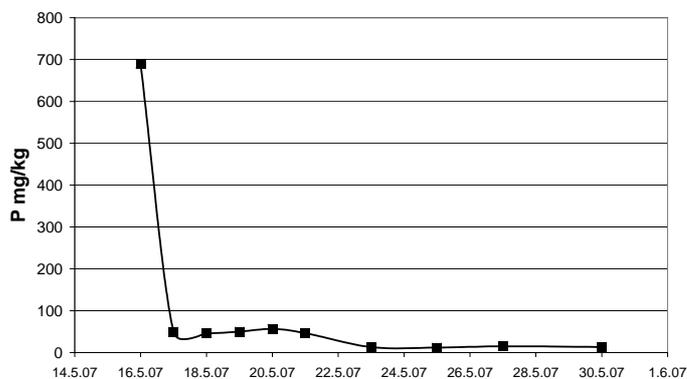
Figure 4. Ortho-P concentration of flowing pig slurry above settled fraction, after gypsum treatment with additives like MgO.
