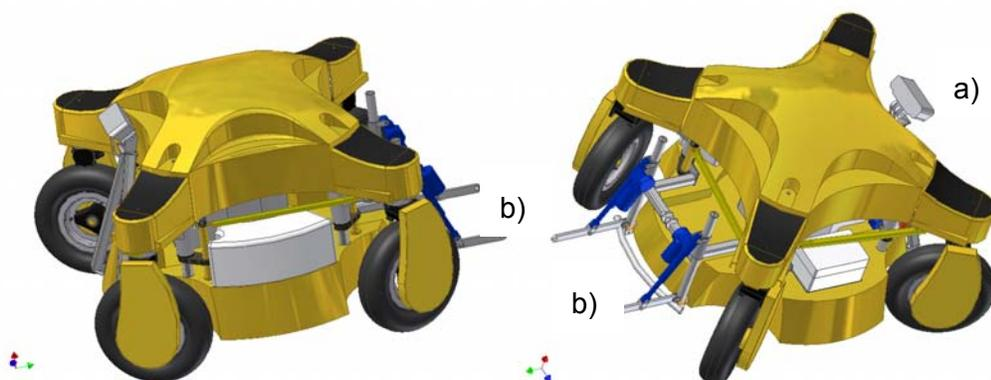
Figure 1. Hortibot design with individual wheel control, 3D row vision system (a), and lift arms (b)
