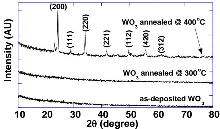
Figure 1. GIXRD spectra of as-deposited and annealed nanostructured  $\text{WO}_3$  thin films.
