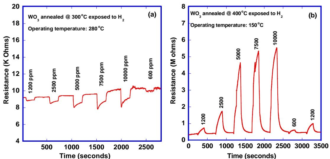
Figure 6: Dynamic resistance curve of nanostructured  $WO_3$  thin films annealed at 300°C (a) and 400°C (b) upon exposure to  $H_2$ .
