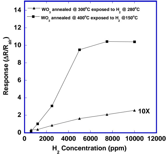
Figure 7: Response upon exposure to H<sub>2</sub> of nanostructured WO<sub>3</sub> thin films. Triangles: film annealed at 300°C, response (x10) measured at 280°C. Squares: film annealed at 400°C (b), response measured at 150 °C.
