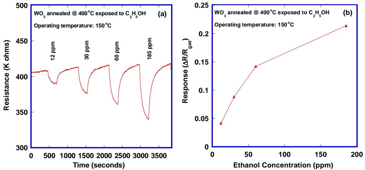
Figure 8: Dynamic resistance curve (a) and Response (b) of nanostructured WO<sub>3</sub> film annealed at 400°C for 2 hours in air, exposed to C<sub>2</sub>H<sub>5</sub>OH.
