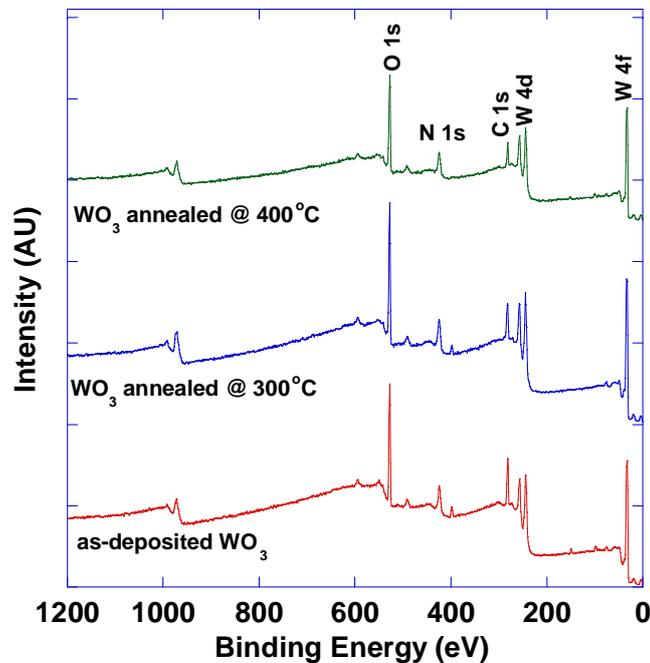
Figure 4: XPS wide survey scans of as-deposited and annealed nanostructured  $\text{WO}_3$  films.
