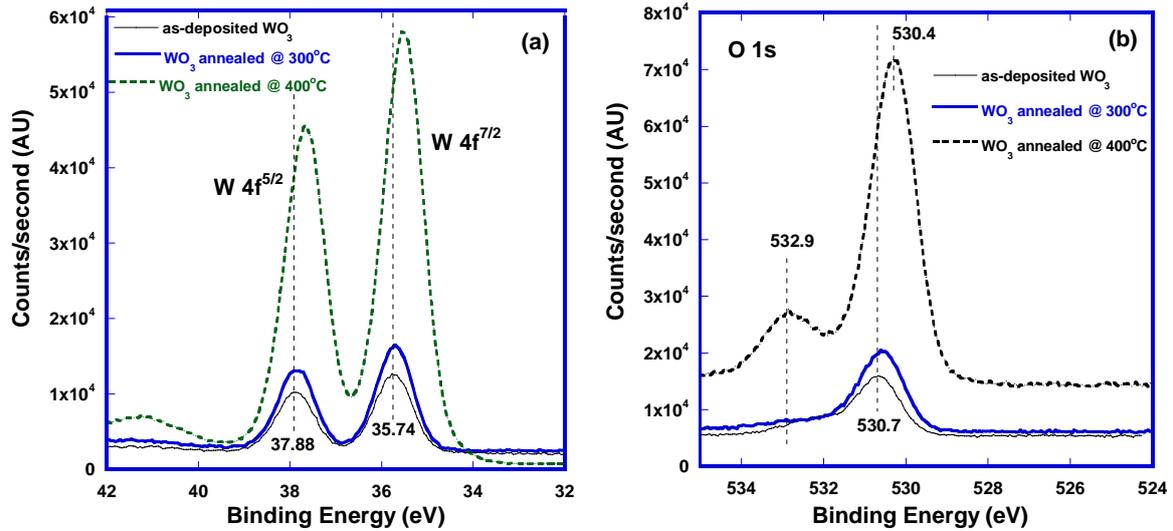
Figure 5: High resolution XPS core level W 4f (a) and O 1s (b) spectra of as-deposited and annealed nanostructured WO<sub>3</sub> films.
