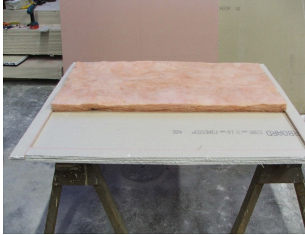
Figure 8: Construction of Test Specimen 6
