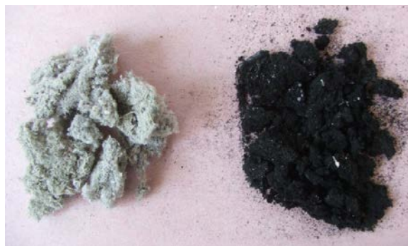
(c) Cellulose Fibre Sample Before and After the Fire Test
