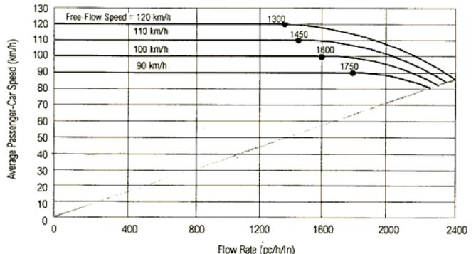
Fig. 3. Speed-flow curve [8]
