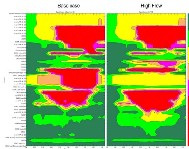
Fig. 9. Speed contour comparison of base case and HF algorithm with natural occupancy set
