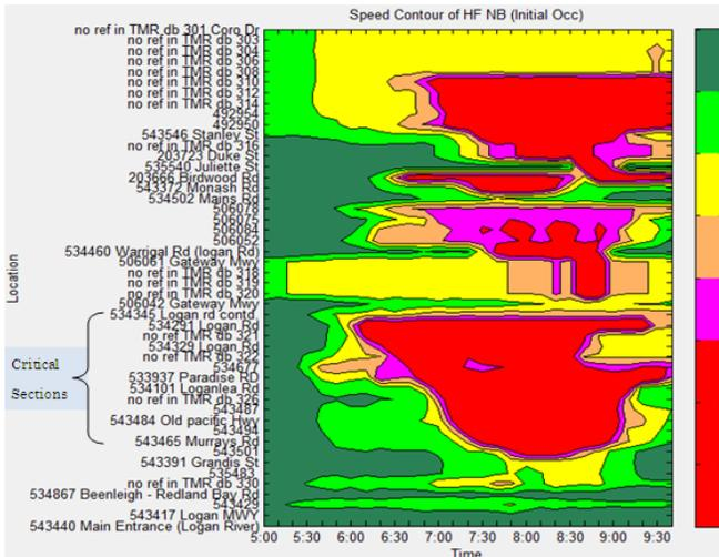
Fig. 7. Speed contour of HF algorithm with initial thresholds and the critical sections
