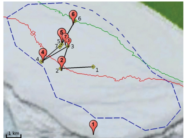
Fig. 10. Execution of the computed path for tracking the centroid of an evolving plume. The initial delineation of the plume to track is given by the dashed line. The waypoints generated by Algorithm 1 are represented by the numbered diamonds. The actual locations where the glider surfaced are given by the numbered droplets. The intended path of the glider (projected to the ocean surface) is the solid line path connecting the numbered diamonds. Image created by use of Google Earth.
