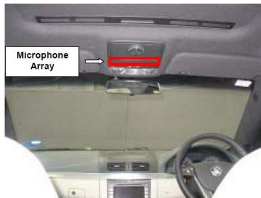
**Figure 1: Position of microphone array inside car cabin.**
