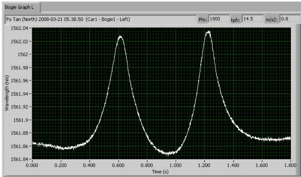
Figure 2: An example of data collected (for one bogie) from a FBG sensor near Fo Tan Station
