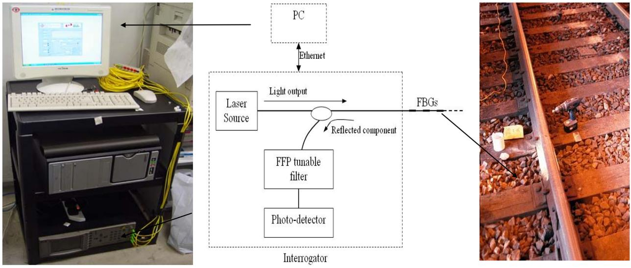
Figure 1: Optical fibre sensing system set-up
