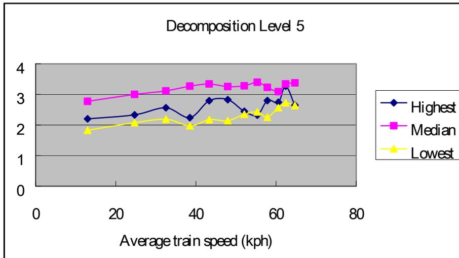
Figure 6: Average peak values of correlations on different train speeds (level 5 signals)
