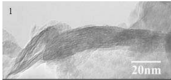
Figure 2. High resolution TEM image of the section area of a stacking clay layers (the area highlighted in Figure 1).
