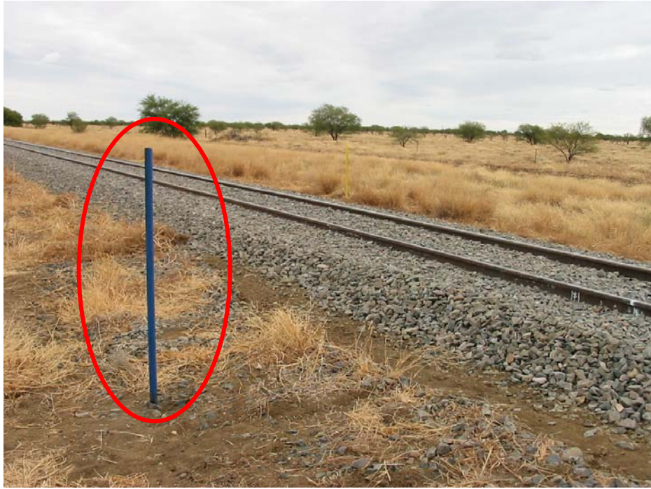
Figure 3.5 Subdivision of Test Area using Coloured Steel Pegs
