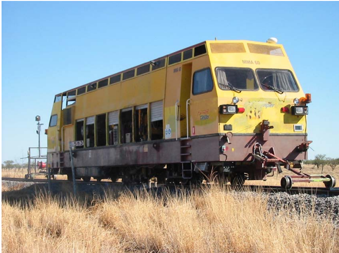
Figure 3.10 MMA 60 – High Production Cycle Tamper
