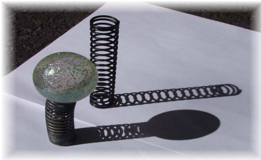
Figure 4-8: Mass on coil compression spring, showing one spring loaded and another identical spring unloaded to illustrate stiffness independence of mass.
