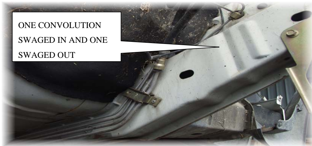
Figure 3-4: Photograph of chassis rail near firewall showing impact weakening convolutions.
