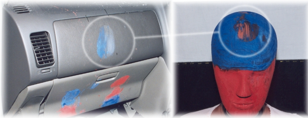
Figure 2-17: Passenger dummy head contact point on dummy and dash.
