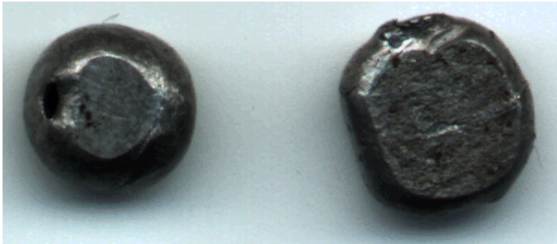
Figure 8-24: Photograph of lead ball after impact with side guide fitted. (LHS is in-line ball, RHS is distal ball.)
