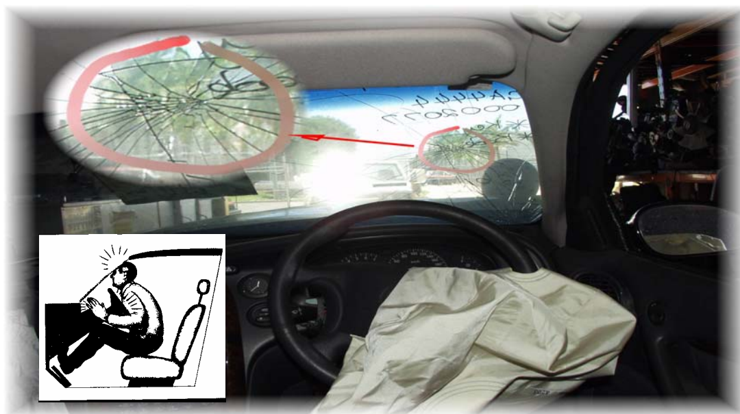
Figure 2-24: Head impact on windscreen despite airbag deployment.
