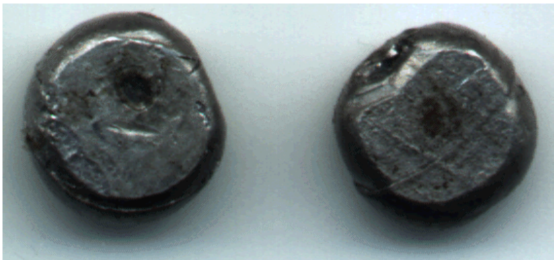
Figure 8-25: Photograph of lead ball after impact with side guide removed. (LHS is in-line ball, RHS is distal ball.)
