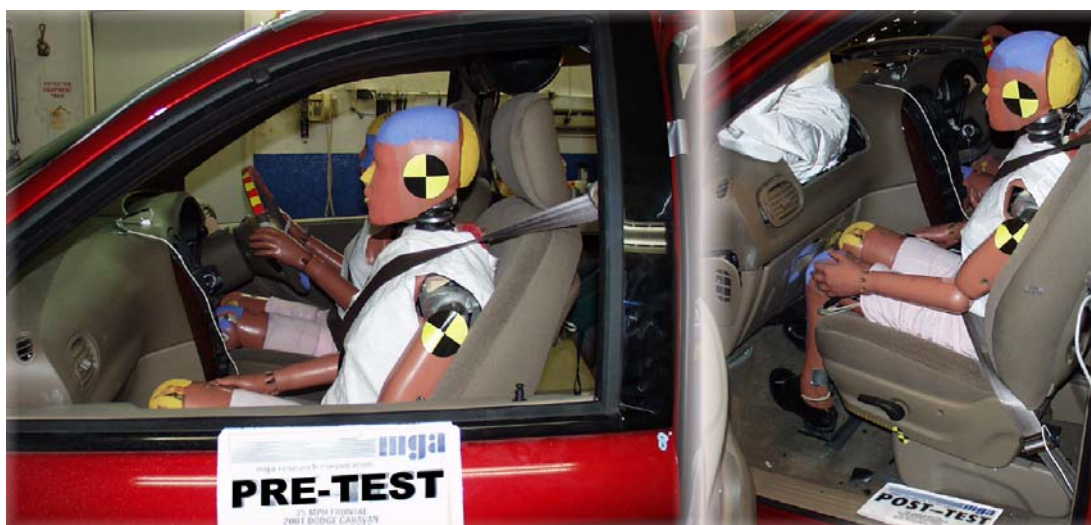
Figure 7-16: Fifth percentile female in 2001 Dodge Caravan (pix mirrored to simulate Australian conditions).
