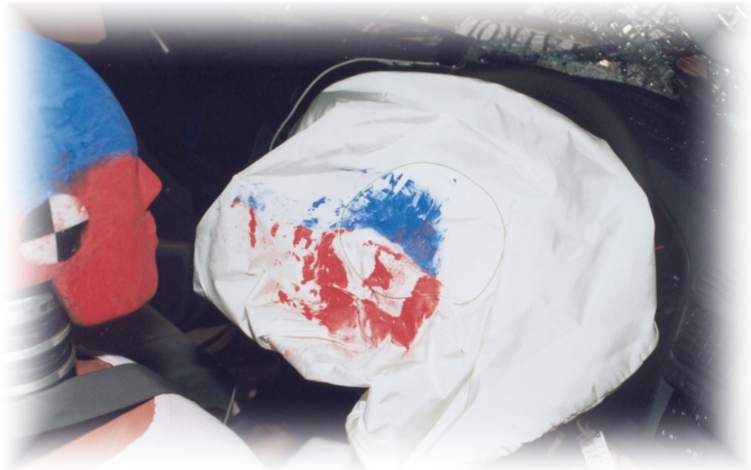
Figure 2-16: Driver dummy contact point on airbag.
