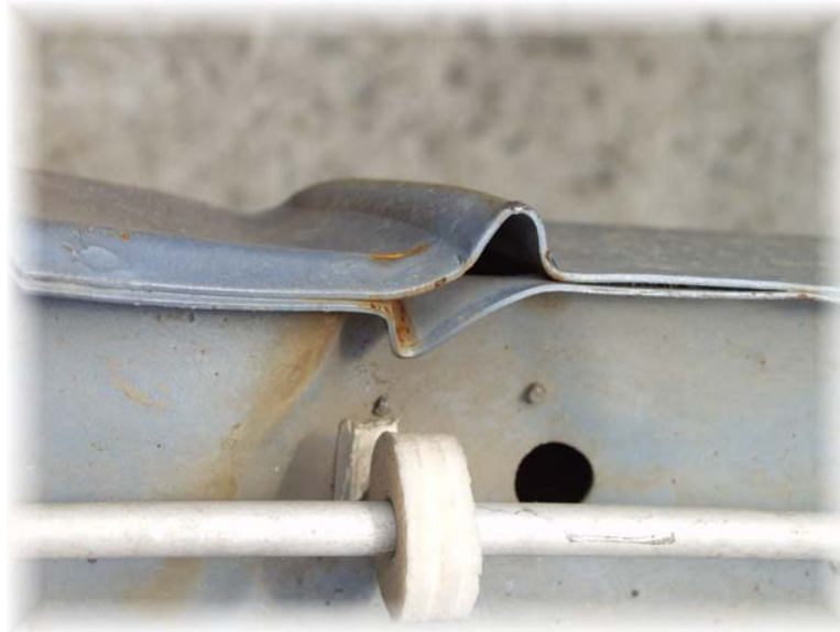
Figure 3-8: Example of local wrinkling in response to a localizing initiator.
