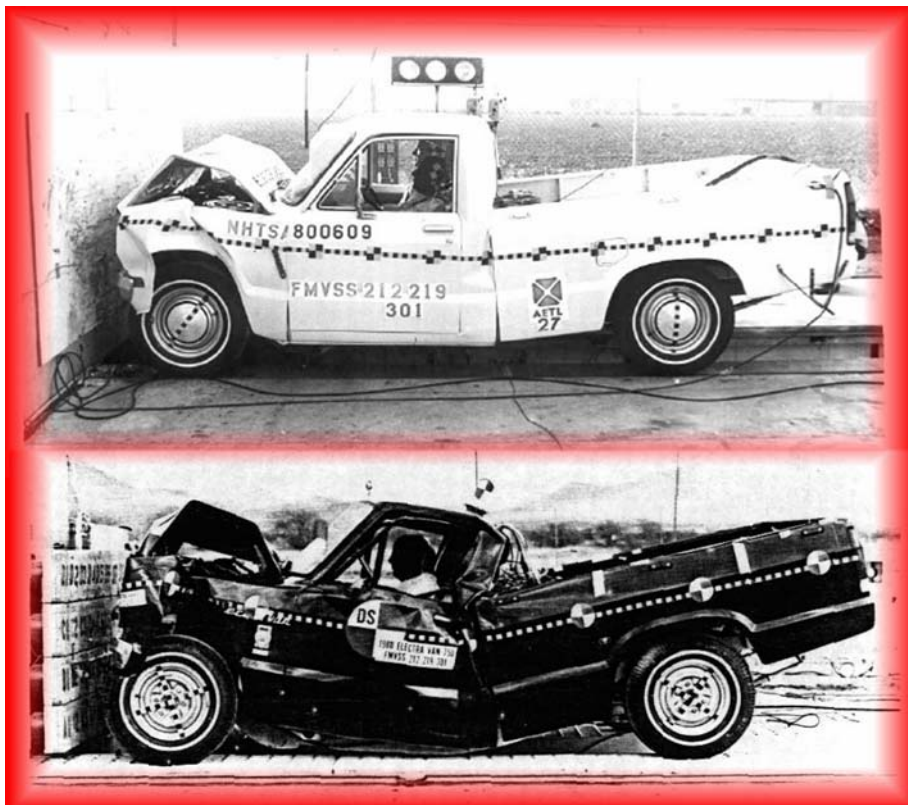
Figure 5-9: Photographs of 1980 Ford Courier after 48 km/h rigid barrier impact. Upper vehicle weight 1427 kg – lower vehicle weight 1982 kg.
