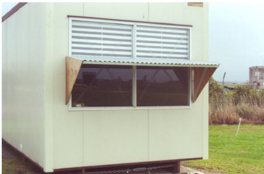
Figure 5.1 - Daylighting Test Building with Vertical Micro-Light Guiding Shade Panel Configuration
