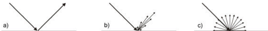
Figure 6.7 - Components of Surface Reflection: a) Ideal Specular; b) Spread Specular; c) Uniform Diffuse
