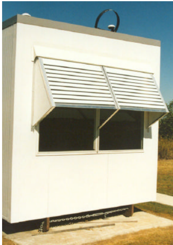
Figure 5.15 - Tilted Micro-Light Guiding Shade Panels Mounted on the Test Building
