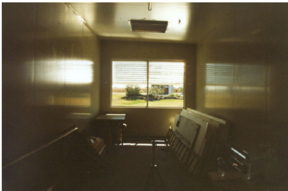
Figure 5.30 - Sunlight Directed into the Eyes of Observers at Solar Noon by the Tilted Micro-Light Guiding Shade Panels
