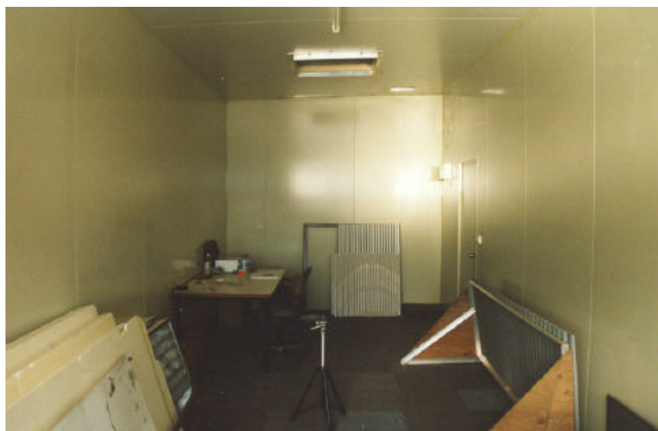
Figure 5.31 - Bright Patch of Redirected Sunlight on the Rear Wall of the Test Building with Tilted Micro-Light Guiding Shade Panels
