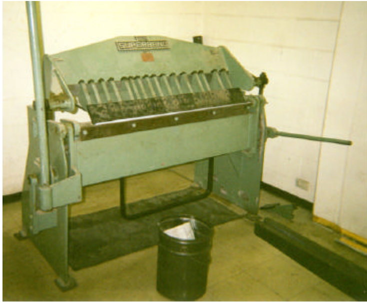
Figure 5.9 - Creating Flat Section Reflectors in a Bending Machine
