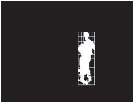
FIGURE 9: The subdivision of the segmentation results in an irregular grid. The ratio of foreground to background pixels in each of the blocks captures the spatial distribution of the body.
