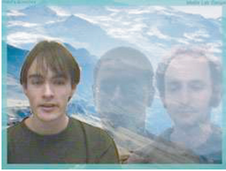
FIGURE 10: Reflexion combines multipoint conference participants in a shared space, a task requiring real-time, visually acceptable segmentation from a desktop PC while leaving enough processing power for audio mixing, object compositing, and other functions (image courtesy Stefan Agamanolis, Media Lab Europe).
