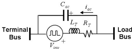
Fig. 10. Single-phase equivalent circuit of DVR.
