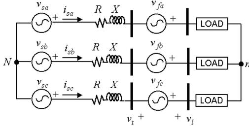
Fig. 1. Schematic diagram of a DVR-connected power system.
