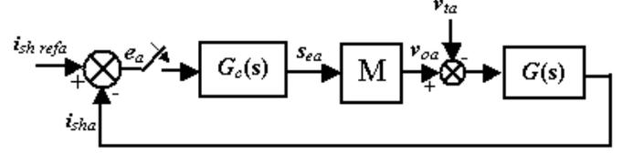
Fig. 7 Current control loop of the DSTATCOM.
