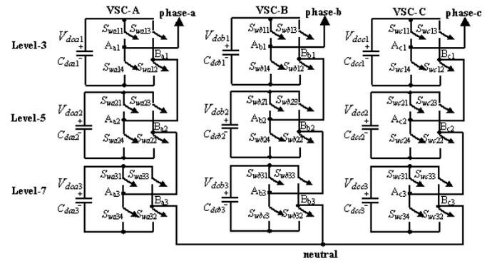
Fig. 4 Cascaded configuration of three-phase seven-level VSC's.
