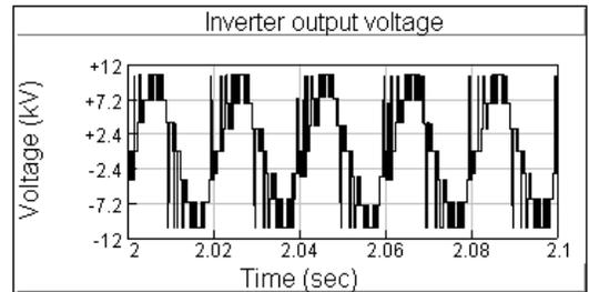
Fig. 14 Inverter output voltage for phase-a.
