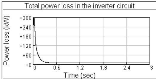
Fig. 16 Total power loss in the three-phase cascaded inverter circuit.
