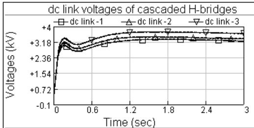
Fig. 15 dc link voltage convergence of the cascaded H-bridges for phase-a.
