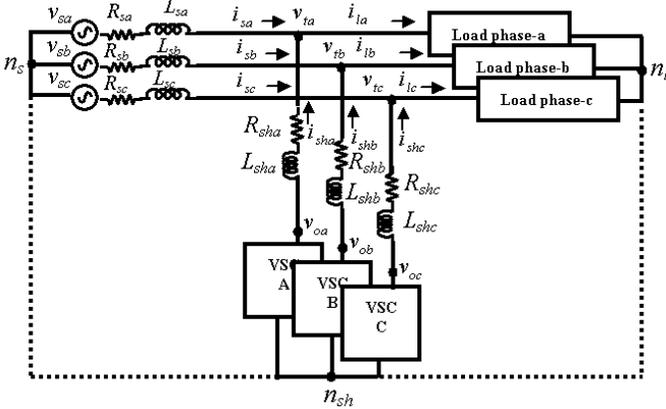
Fig. 6 Shunt compensation of three-phase four-wire distribution system.
