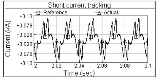
Fig. 13 Shunt current tracking characteristics of phase-a.
