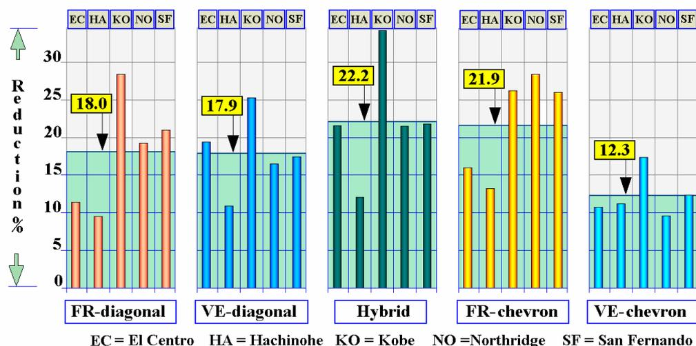
Figure 5: Average reduction in tip deflection for all five types of damping systems.
