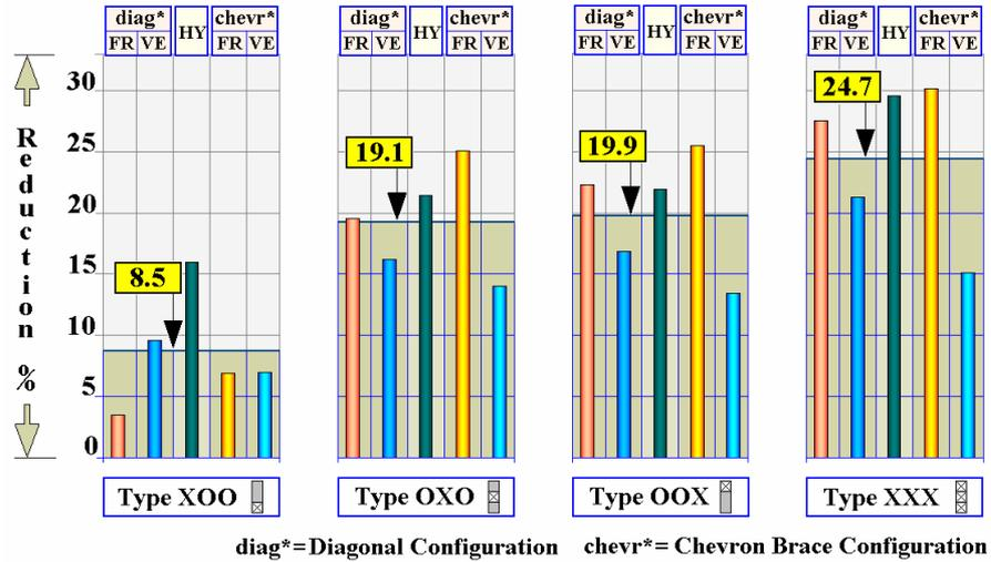
Figure 6: Average tip deflection reductions (under all five earthquakes) for different damper location.
