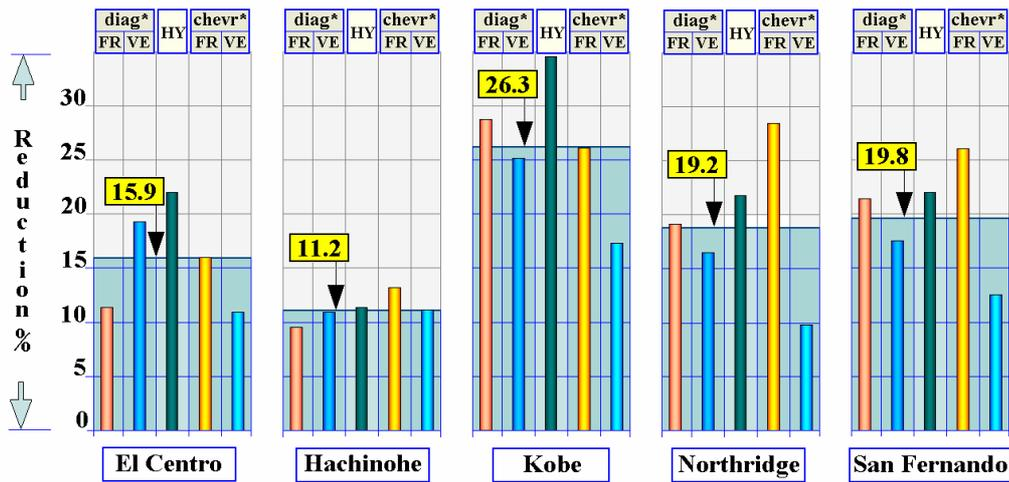
Figure 7: Average tip deflection reductions (for all five types of damping systems) under each earthquake.
