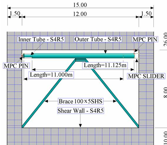
Figure 4: Structural details of friction damper – chevron brace configuration.
