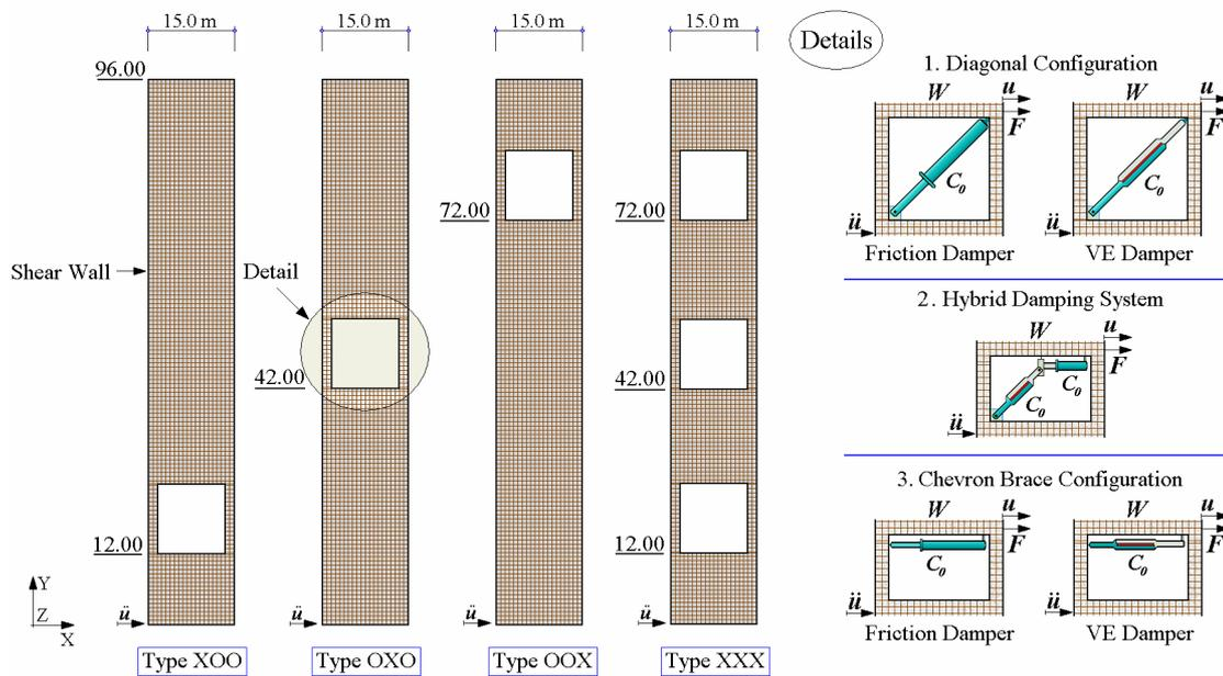
Figure 1: Placement of dampers within shear walls.
