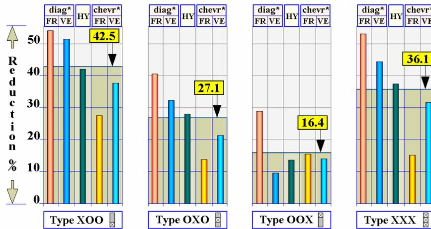
Figure 9: Average tip acceleration reductions (under all five earthquakes) for different damper location.
