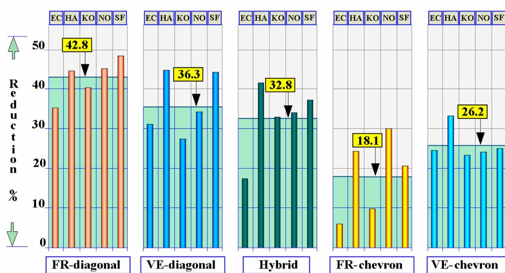
Figure 8: Average reductions in tip acceleration for all five types of damping systems.
