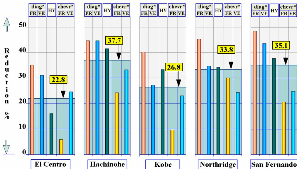
Figure 10: Average tip acceleration reductions (for all five types of damping system) under each earthquake.
