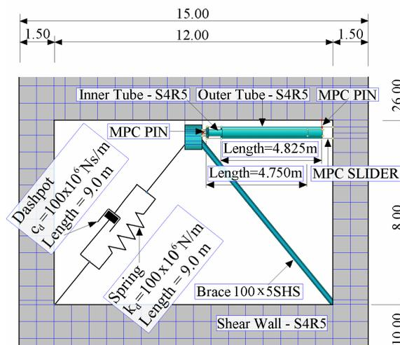
Figure 3: Structural details of hybrid damping system.
