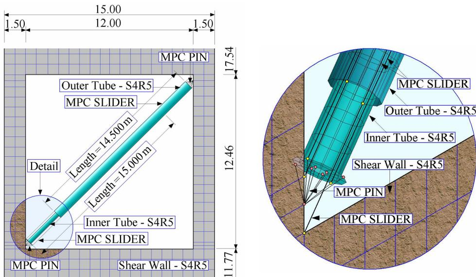
Figure 2: Structural details of friction dampers – diagonal configuration
