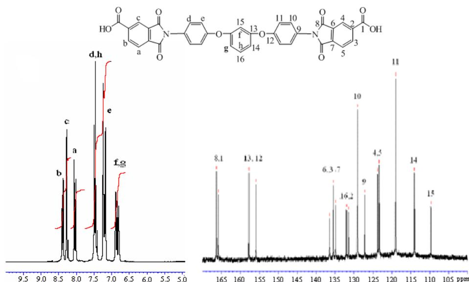
**Figure 3.** <sup>1</sup>H NMR and <sup>13</sup>C NMR spectra of diimide dicarboxylic acid monomer
