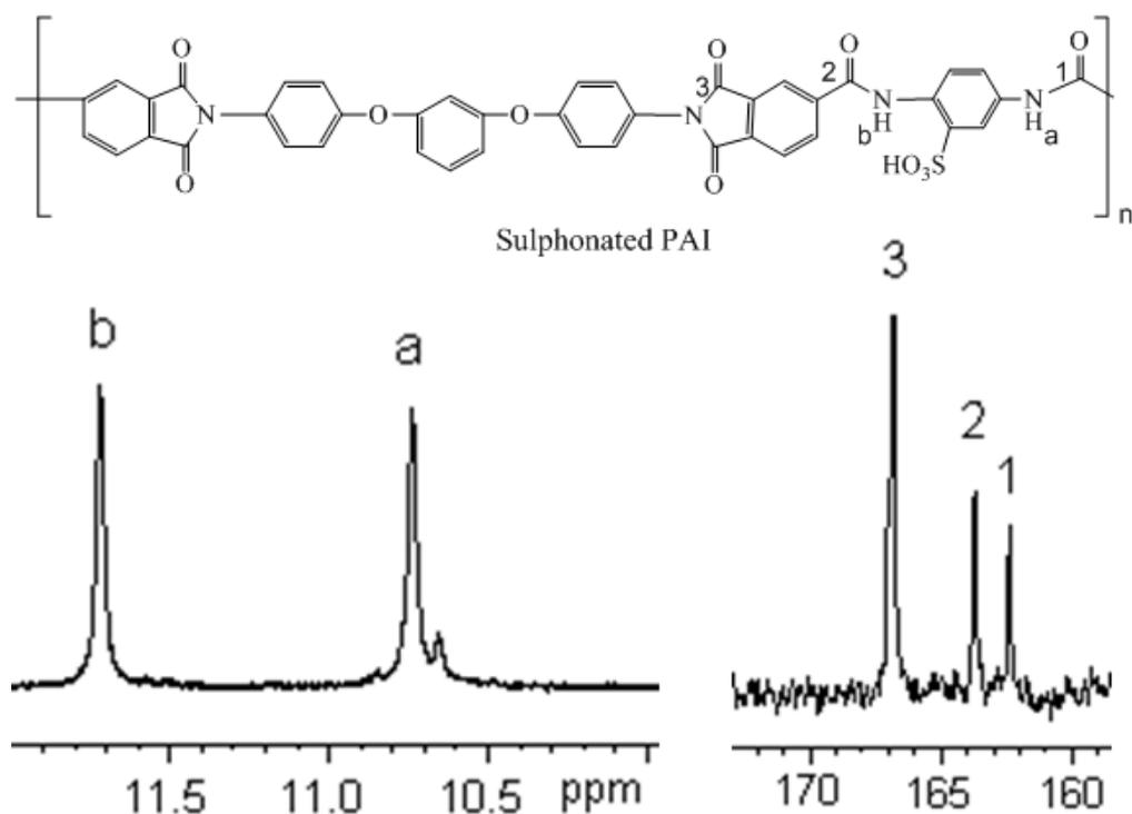
**Figure 5.** Main peaks of  $^1\text{H}$  NMR and  $^{13}\text{C}$  NMR spectra of sulphonated polyamideimide.
