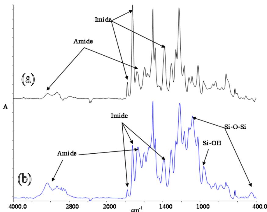
**Figure 7.** FTIR spectra of polyamideimide (curve a) and polyamideimide/silica hybrid (curve b) thin films.
