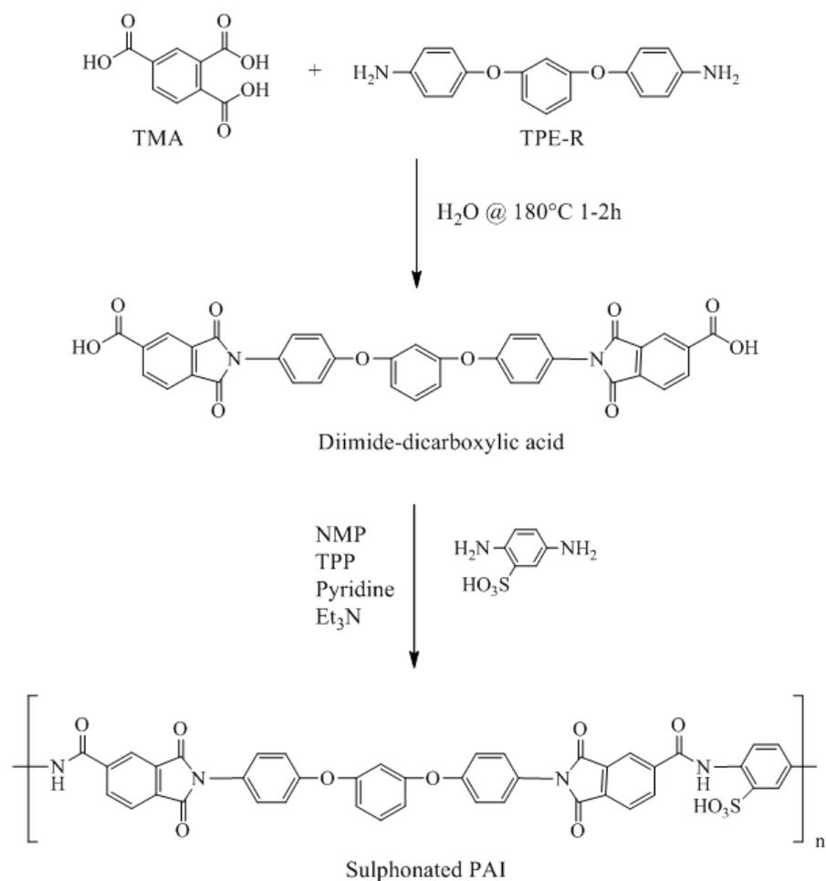
**Figure 1.** Synthesis scheme of sulphonated polyamideimide
