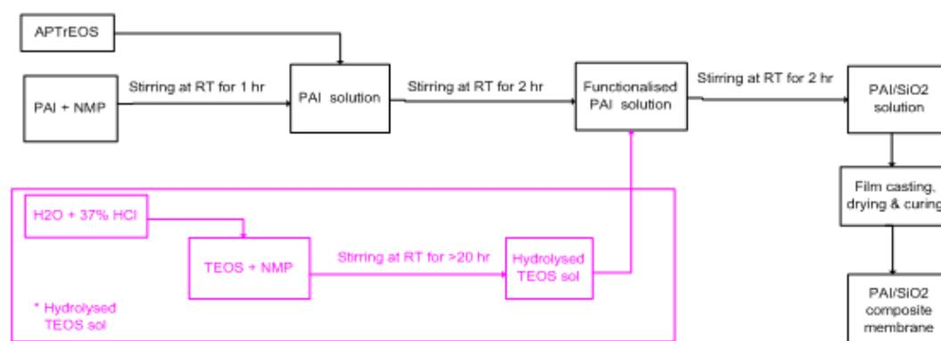
**Figure 2.** The preparation process of polyamideimide/SiO<sub>2</sub> hybrid membrane
