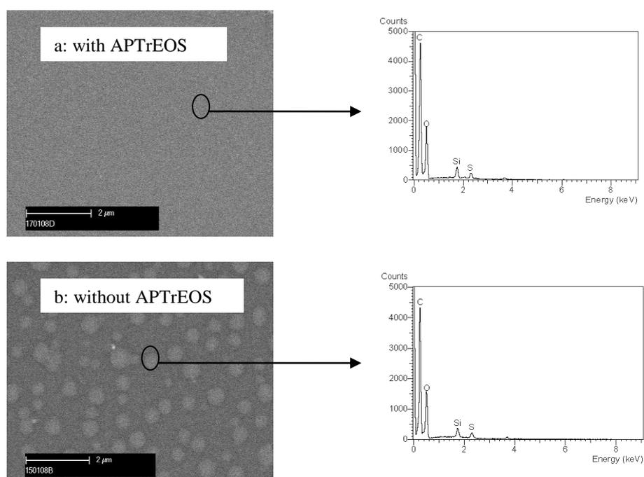
**Figure 9:** SEM images and EDS spectra of polyamideimide/silica hybrid film samples (all containing 7 wt% SiO<sub>2</sub>, a: with APTreOS, b: without APTreOS).
