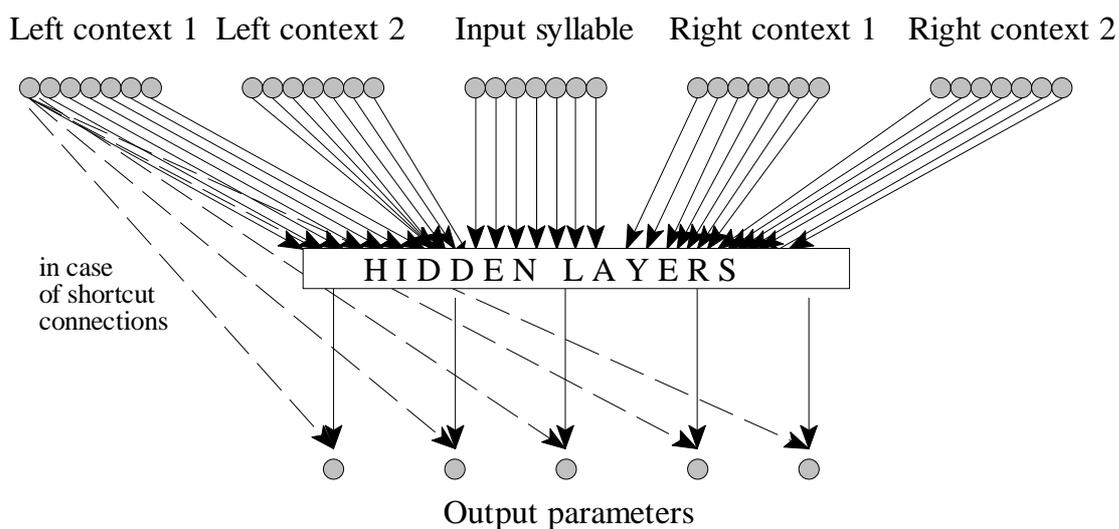
**Figure 2** General structure of the network: 35 real input nodes, 5 real output nodes, one or two hidden layers. In case of shortcut connections all the input nodes are directly connected with all the output nodes.
