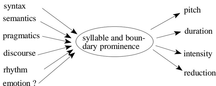
**Figure 1** Structure of the prominence-based synthesis system. The transition from prominence to pitch and duration values is carried out by a neural network.
