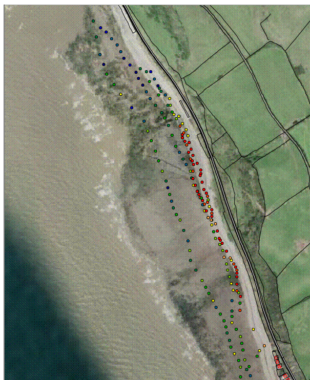
Figure 2.2: 137 Cs activity measurements along a 1km section of beach from the follow-up survey, 18 th March 2000.
