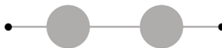
Figure 5.8 Mask pattern used for photolithography of the inlet/outlet ports is shown in black. This mask was aligned with the existing pattern from the first etch, shown in grey.
