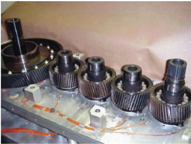
Figure 6: Baseline test hardware during installation.
