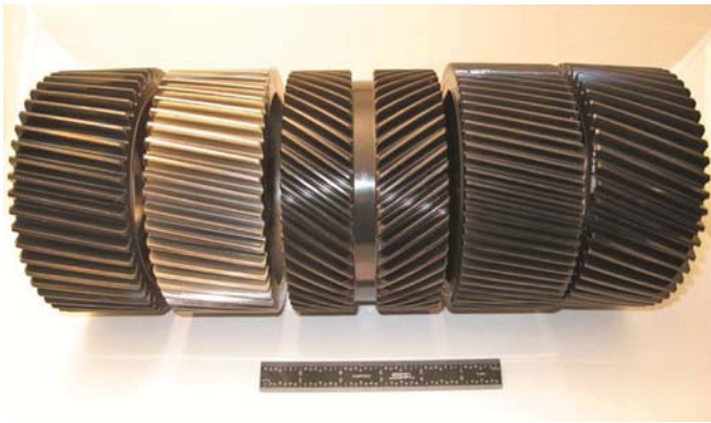
Figure 5: Photograph of input gear designs. Baseline, baseline + ISF, double helical, fine pitch, and increased helix angle.
