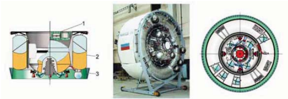
Figure 1 – The Briz-M upper stage is composed of a central engine surrounded by a donut-shaped auxiliary propulsion tank, which is ejected part-way through a nominal mission. The Briz-M stage described in this paper failed with the donut-shaped tank still attached and containing substantial amounts of fuel.
