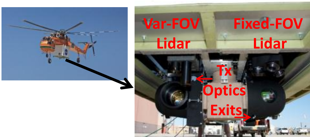
Figure 10: Instrumentation pod installed on Erickson Aircrane helicopter (left) lifting off from NASA-Dryden and en-route to Edwards AFB test range carrying the ALHAT instrumentation pod with pod belly doors closed and the lidars retracted. The right image shows the pod doors open and lidars deployed with protective aerodynamic shrouds on each and laser exit apertures noted.
