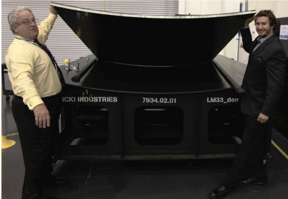
Figure 1.—Photograph of cured 1/16 th arc segment panel and the tool it was molded on.
