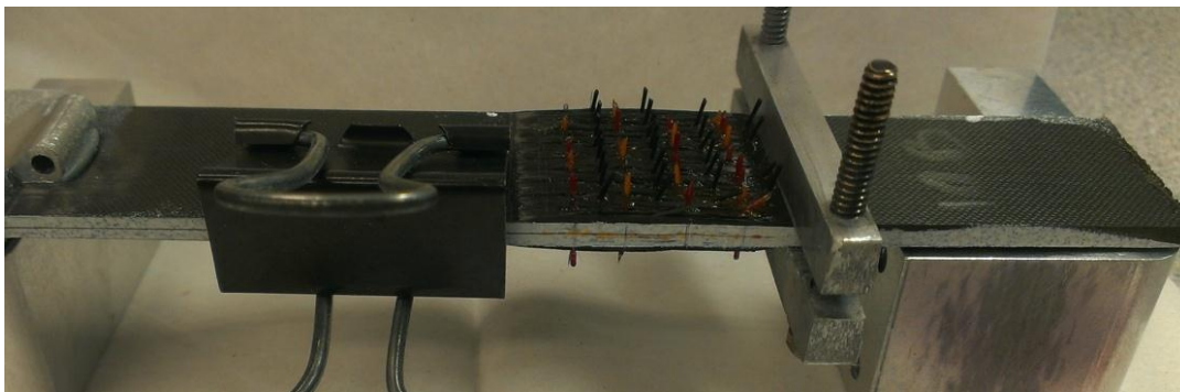
Fig. 31. Sealing resin visible on edge of specimen 10B
