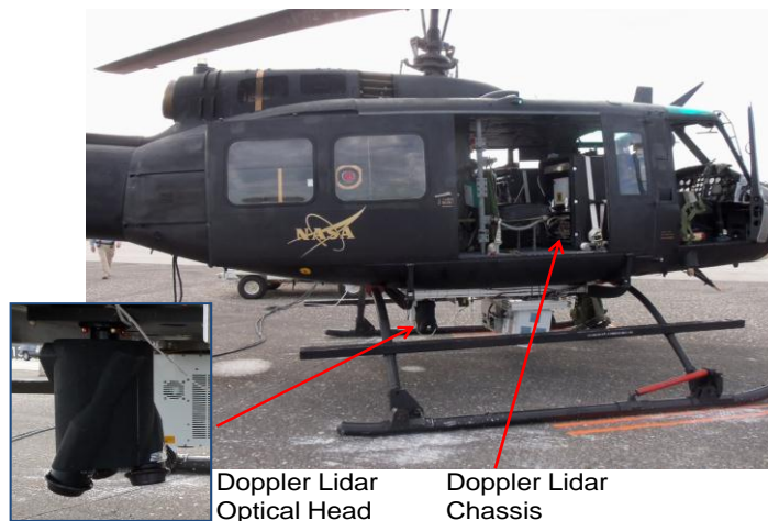
Figure 5. Helicopter flight test of Doppler lidar at NASA-KSC in 2012, along with other sensors and landing avionics developed under ALHAT project.
