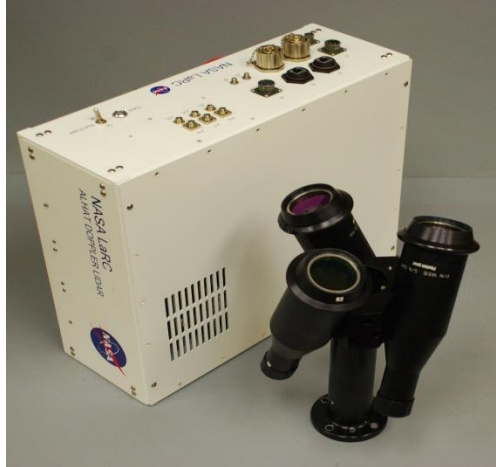
Figure 4. Prototype Doppler lidar system consisting of an electronic chassis and an optical head. All the lidar components, including transmitter laser, receiver, and real-time processor, are housed in the electronic chassis. The optical head, housing the three transmit and receive lenses, is rigidly mounted to the platform body with a clear view of the ground and connected by an armored fiber cable to the electronics chassis.
