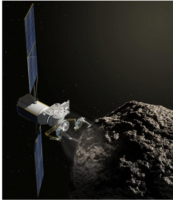
Figure 8: SEP-based excursion vehicle concept for a human NEA mission (image credit: NASA/AMA, Inc.).
