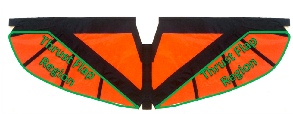
Figure 15. Wing planform showing the thrust flap region. When the thrust flap changes direction a peak occurs in the body vertical acceleration curve.
