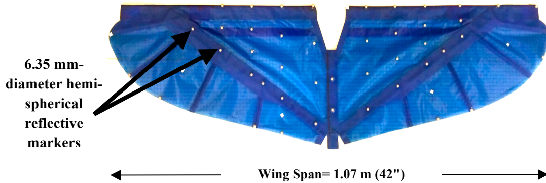
Figure 5. Wing Reflective Markers Placement. Markers were distributed over both wings to balance the weight and they were placed asymmetrically to aid with tracking and post processing.
